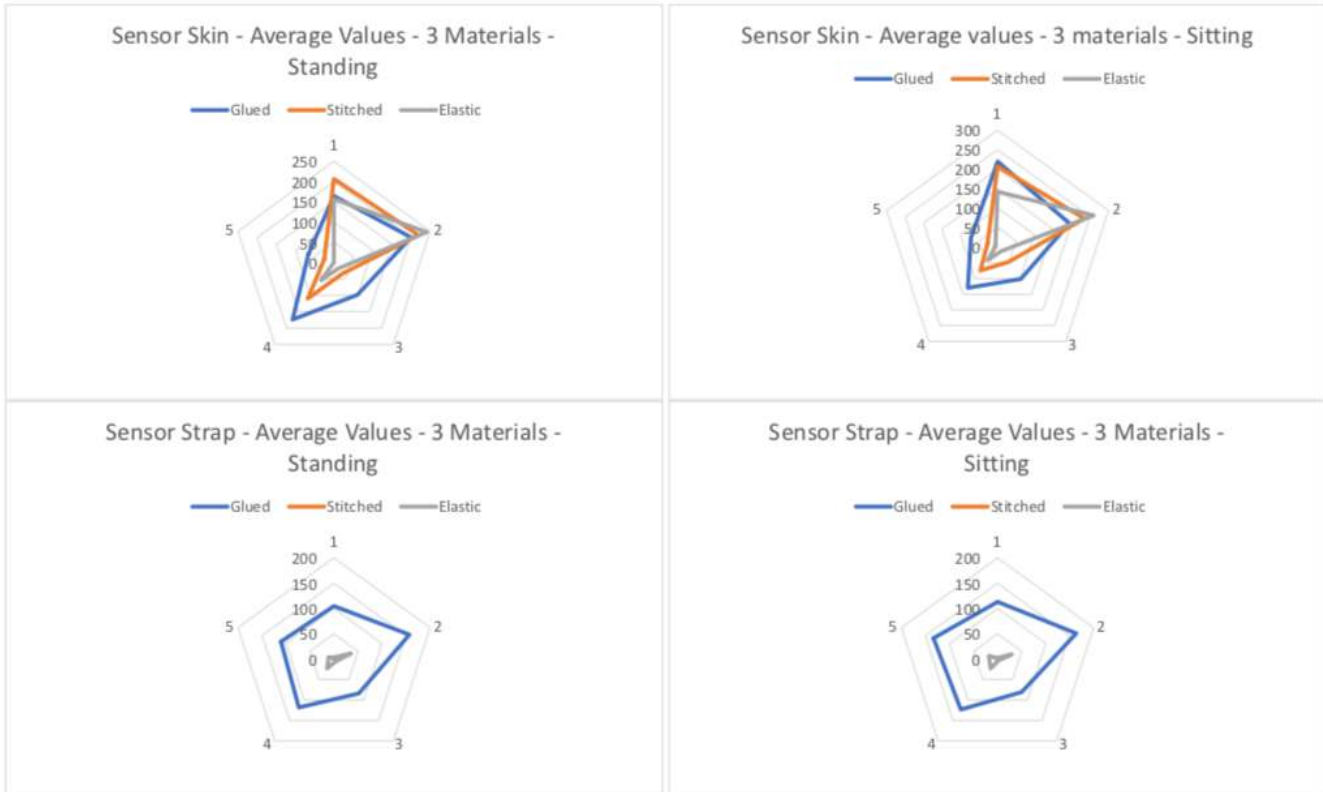
Figure 4 – Comparing three strap systems (Glued, Stitched and Single Elastic) – Strap length 711 mm
